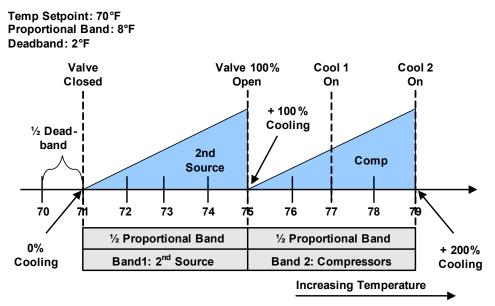
**Minimum Chilled Water Temperature**—This feature permits the user to select the minimum chilled water temperature that allows simultaneous operation of the second cooling source (chilled water control) and compressor control. This feature is enabled in the Service menu under Setpoints, parameter Minimum CW Temp.
